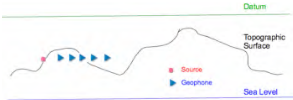
Figure 37. Simple Topographic Schematic After Correction to Source Position
