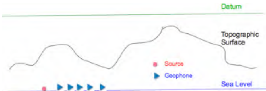
Figure 38. Simple Topographic Schematic After Correction to Sea Level
