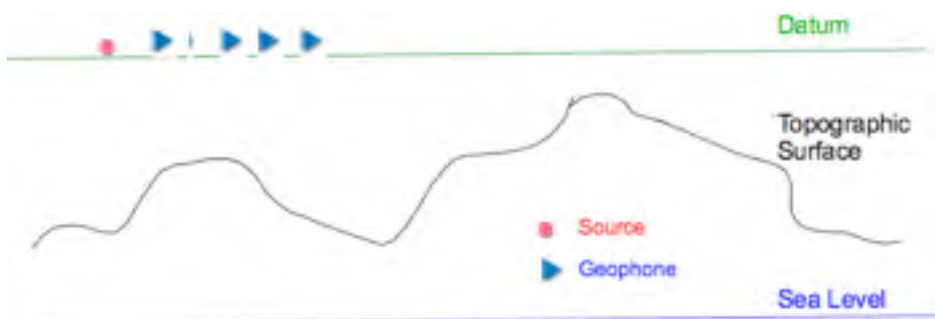
Figure 39. Simple Topographic Schematic After Correction to Datum Elevation
