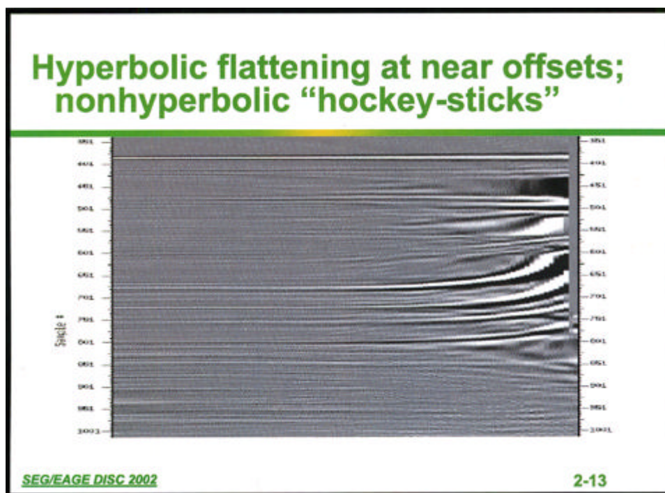
Figure 11-4. After Leon Thomsen DSC 2002. Typical hockey stick character after application of NMO using the usual stacking velocity equation without the anisotropic term.
