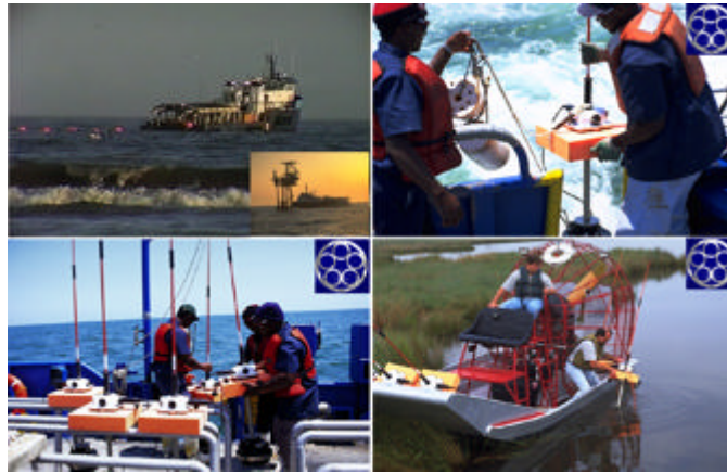
Figure 8-19. This figure shows boxlike ocean bottom receivers being deployed overboard (bottom left and top right) in both deep and shallow marine environments. The top left composite demonstrates that source boats can operate close to shore and platforms.
