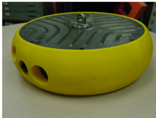
Figure 8-20. Fairfield Industries' latest ocean bottom recorder contains four phones and all the electronics necessary to record source-responses.
