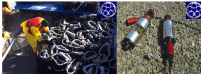
Figure 8-18. Ocean bottom layout and acquisition. This figure shows the cables and sensors used to acquire data from ocean bottom cables.
