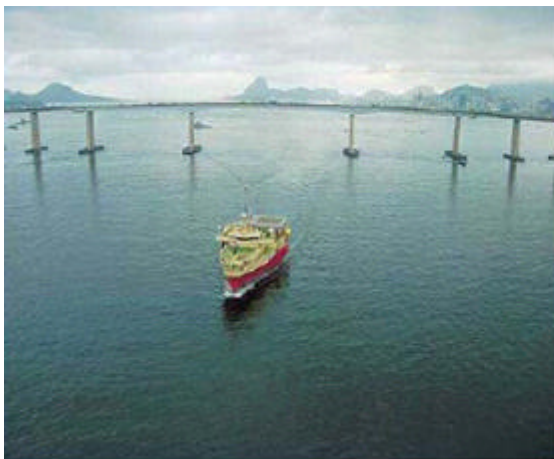
Figure 8-12. Petroleum Geo-Services (PGS) boats in operation. Note the towed streamers and the triangular shape of the Ramform boats.
