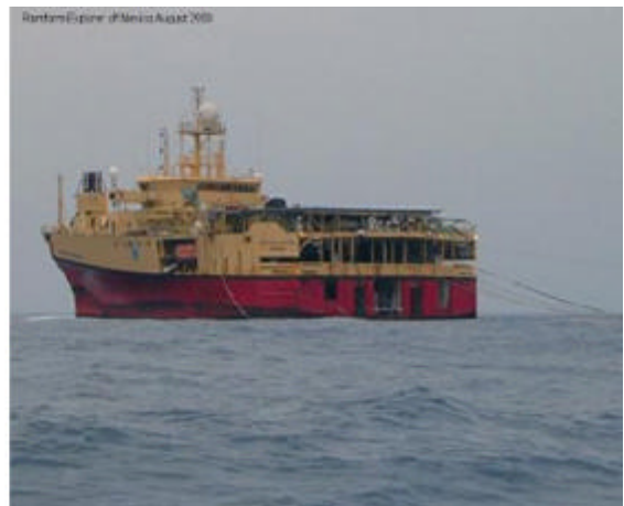
Figure 8-12. Petroleum Geo-Services (PGS) boats in operation. Note the towed streamers and the triangular shape of the Ramform boats.
