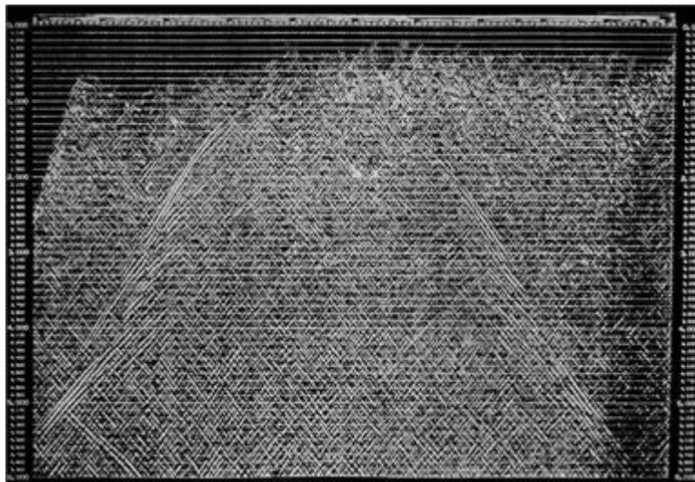
Figure 3-45. Stack of the data using an assumed dip of 37.5 degrees. At the bandwidth of these data the effect is to stack everything between 30 and 45 degrees of dip.
